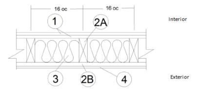
GYPSUM BOARD (Interior): Two layers USG Firecode<sup>®</sup> C Core, complying with ASTM C1396, min. 5/8 in. thick, 4 ft. wide applied vertically, fastened to framing. Face layer joints staggered with base layer and covered with paper tape and joint compound.
