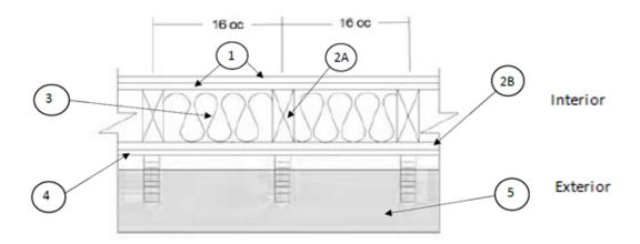
1. GYPSUM BOARD (Interior): Two layers Type X complying with ASTM C1396 min. 5/8 in. thick, 4 ft. wide applied vertically, fastened to framing. Face layer joints staggered with base layer and covered with paper tape and joint compound.
